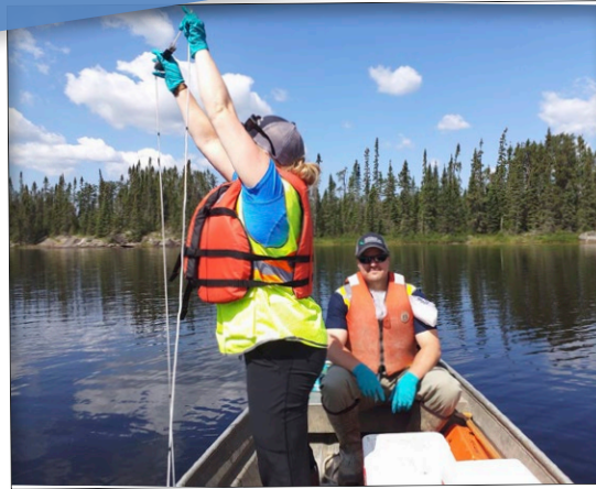
Using a kemmerer to collect mid depth water samples at a pond in the AOI.
